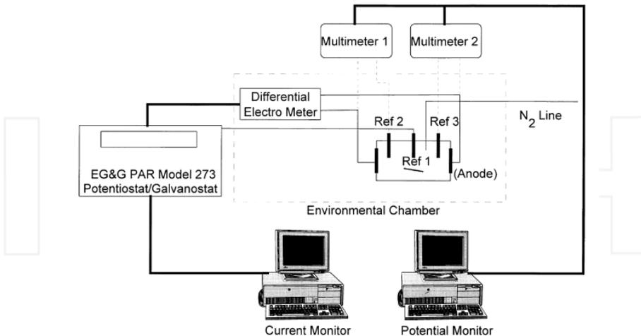
**Figure 2.** Schematic diagram for the galvanic cell set-up [8].
