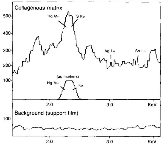
Fig. 8. - Corresponding X-ray spectrum of the mercury M- $\alpha$  peak compound with sulphur K- $\alpha$ . Silver and tin if present would be identified as L- $\alpha$  lines at 2.98 and 3.43 keV, respectively.
