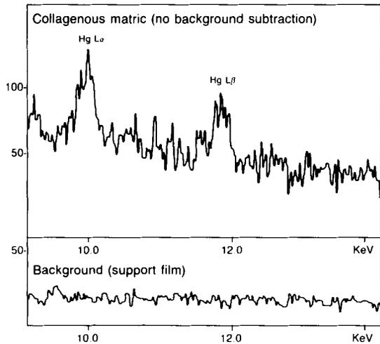
Fig. 7. - X-ray spectrum of representative area of the connective tissue matrix showing mercury L- $\alpha$  and  $\beta$  peaks.
